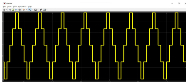
Fig. 7. Current Output When Four MLC Module Circuits Are Operating Simultaneously
