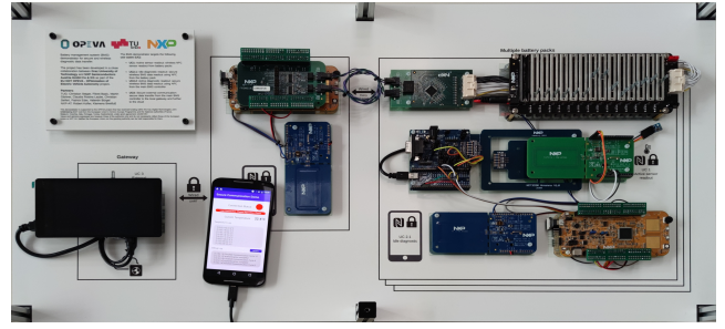
Fig. 3. Wireless BMS demonstration build for battery passport readout.
