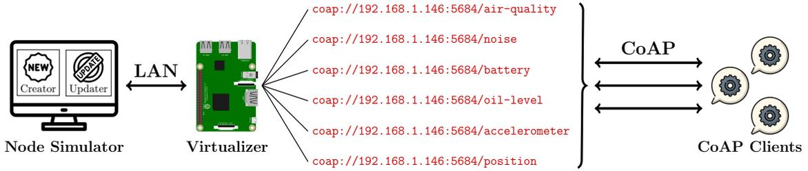
Fig. 6: Setup for the experimental evaluation of the proposed virtualization architecture, with the Virtualizer hosted on a RPi3. The experimental performance evaluation has also been carried out hosting the Virtualizer on a laptop.
